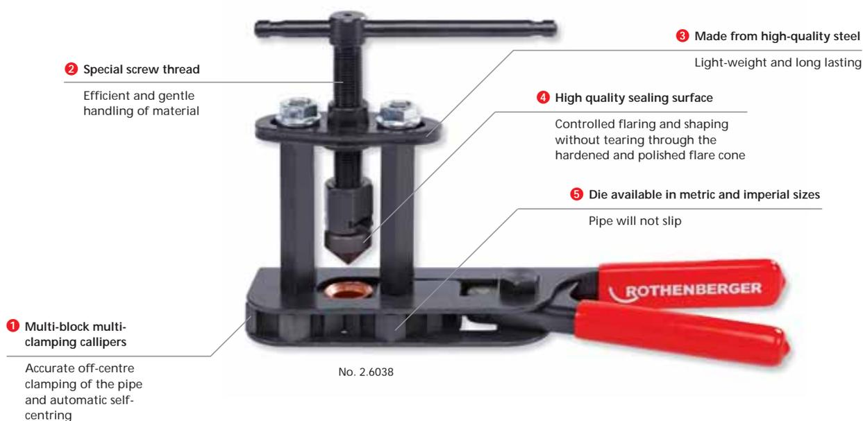
ROFLARE sets include: ROFLARE Basic Unit with integrated attachments
