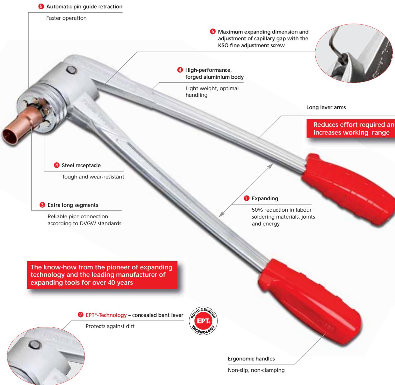
The know-how from the pioneer of expanding technology and the leading manufacturer of expanding tools for over 40 years
